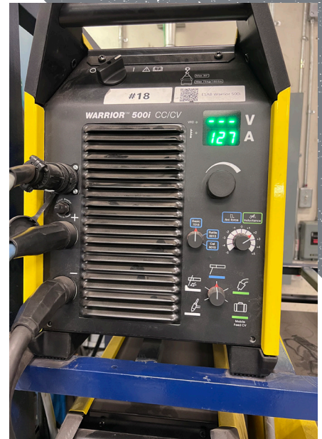
The Warrior features an intuitive color-coded interface (blue for Stick, green for MIG or flux cored) that links processes to their associated controls, such as arc force and inductance.
